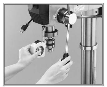
Figure 27. Actual stop depth being measured.
